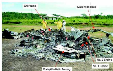
Figure 6.9: Photograph of the wreckage looking due south, showing the extent of fire damage and identifying some of the aircraft features.
